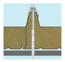
ROOF ASSEMBLY In order to assure the right water outflow as well as to avoid oxidation phenomenon on metallic supports, the panels must be assembled with a slope not lower than 7%.
