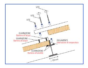
METECNO ITALIA recommends to ask the preparation for the end-lapping in order to avoid any infiltration into the insulation or inside the building.
